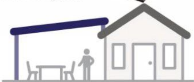
Flyover style roof with roof penetration brackets
